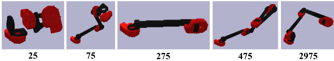
Fig. 5. Validation arrangements for the goal [0.2, 0.2, 0.2] . By episode 475, the network is able to produce an arrangement that can reach the desired goal position. However, by the end of the training the network has learned that only two links are needed to reach the goal instead of three.
