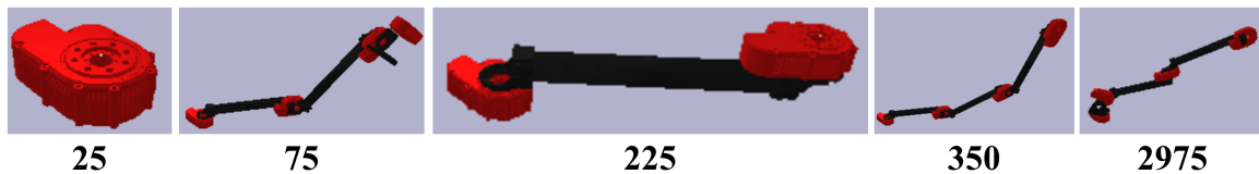
Fig. 8. Validation arrangements for the goal [0.5, 0.5, 0.5] . The network appears to learn at an early point in the training that several links will be required to reach this goal position. This can be seen in the longer arrangement shown at episode 75. By the end of the training, the network still uses the same number of links as it did at episode 75, but it has moved the bracket to be earlier on in the arrangement which allows the arrangement to be more flexible.
