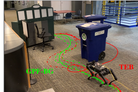
Fig. 1: Unitree A1 quadruped navigates an unknown, constrained environment. Depicts robot navigation paths for GPF-BG (green) and TEB (red).
