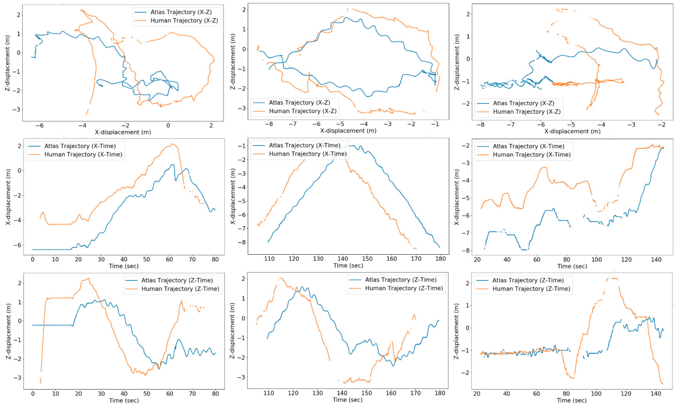
Fig. 6: Motion Capture trajectories for human target and Atlas while performing Track-and-Follow Behavior. Each column represents a different experiment. The first two columns were obtained on flat-ground, and the last column on rough terrain.
