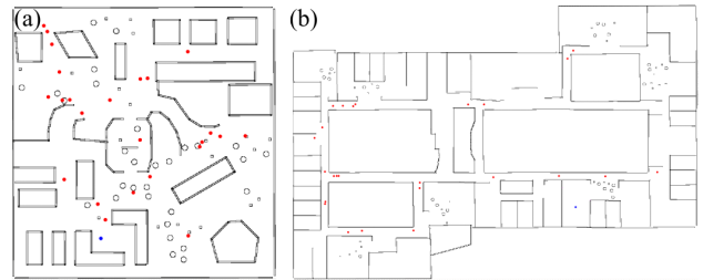
Fig. 6. Campus (left) and Office (right) World in STDR simulator, with dynamic agents (red) and ego-robot (blue).
